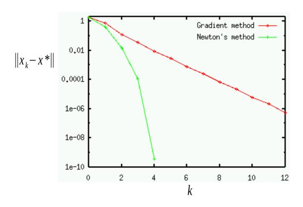
Newton's method much faster than gradient method
