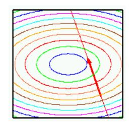
For Newton's method: If the quadratic model is good, then step is good, then take *full step* with  $\alpha_k = 1$
