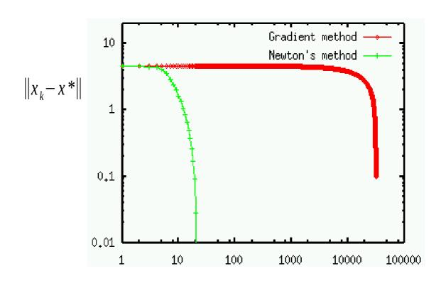
Newton's method **much** faster than gradient method
