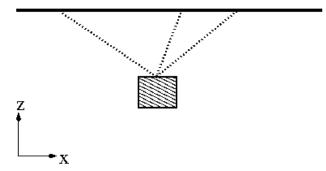
Each spring has a rest length of  $L_0 = 20$ cm, and extending (or compressing) spring i, i = 1...3 to a length  $L_i$  requires an energy of  $E_{\text{spring},i} = \frac{1}{2}D(L_i - L_0)^2$  where the spring constant for all three springs equals  $D = 300 \frac{N}{m}$ . On the other hand, the potential energy of the body is  $E_{\text{pot}} = mgz$  where the body's mass is m = 500g, the gravity constant is  $g = 9.81 \frac{m}{c^2}$ , and z is the vertical coordinate of the body's position.
