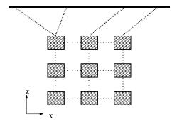
The four springs at the top are suspended from the ceiling at positions (x, z) = (-20cm, 0cm), (-5cm, 0cm), (7cm, 0cm) and (15cm, 0cm) and have rest lengths of  $L_0^{\text{top}} = 20\text{cm}$ . The 9 bodies are connected with 12 springs of rest lengths  $L_0^{\text{between}} = 5\text{cm}$ . All springs are attached to the centers of the sides of the bodies, which all have a size of  $2\text{cm} \times 2\text{cm}$  and have a mass of m = 500g.
