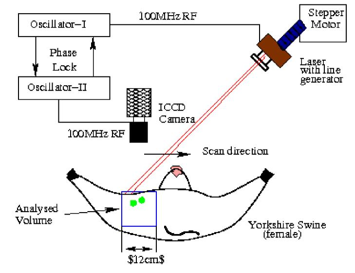
Experimental setup, a widened laser line scans the pig at 6 locations
