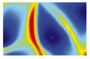
Visualizations of oil reservoir simulations at various stages in an optimization. Pumps, represented by asterisks, push oil toward wells, represented by small white circles, that draw oil from the ground. Blue areas indicate areas of high water concentration. Brown areas indicate areas of high oil concentration. By the end of the simulations, there is not much oil left in the reservoir, and what is left has been swept toward the wells.
