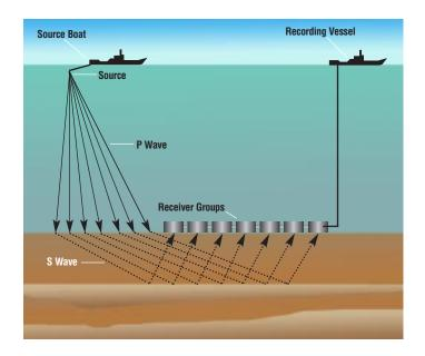
Illustration of soundings being taken on the ocean. Sound waves are projected from a ship, pass through the water, and are altered by the rock in the ocean floor. The echo from this process is picked up by receivers on the ocean floor or seismic monitoring platforms. It can be translated into information about things like the type, density, and permeability of the rock and the amount of oil contained within. These soundings are taken over and over from different positions for a single area.
