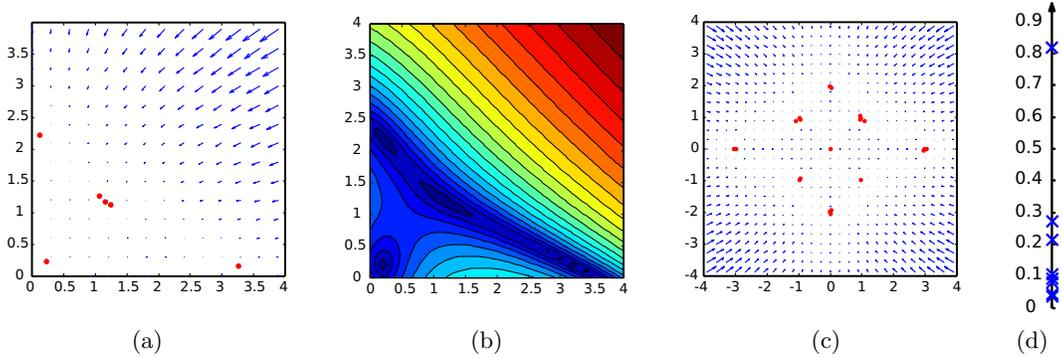
**Figure 3:** (a) A plot of the Lotka-Volterra competitive equations with a small shift in the coordinates represented by vectors, with the detected fixed points shown. (b) The contour plot of the norm of the function. (c) The Lotka-Volterra equations with the upper right quadrant tiled and reflected appropriately. (d) The well diagram for (c).
