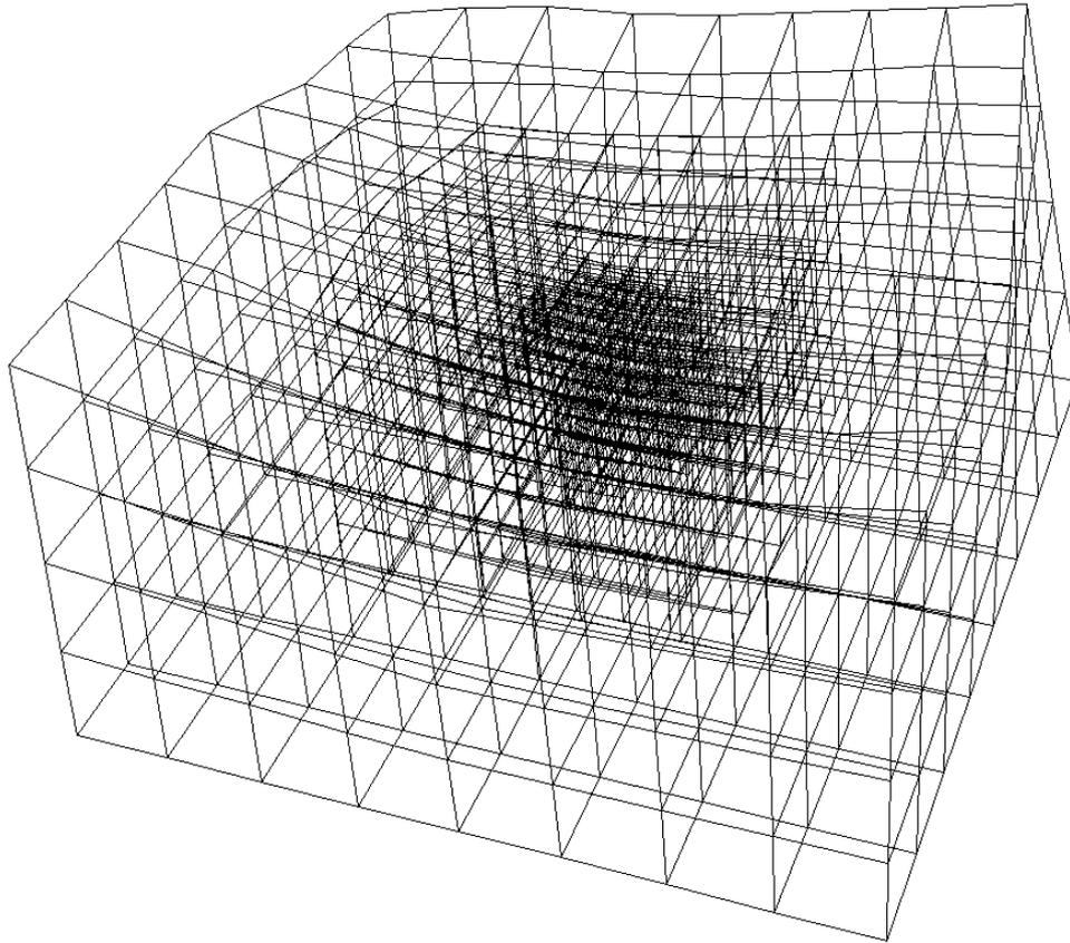
Mesh used to discretize the unknown parameter
