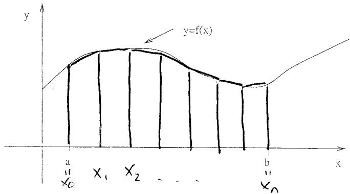
divide  $[a, b]$  into  $n$  parts of length  $\Delta x = \frac{b-a}{n}$
