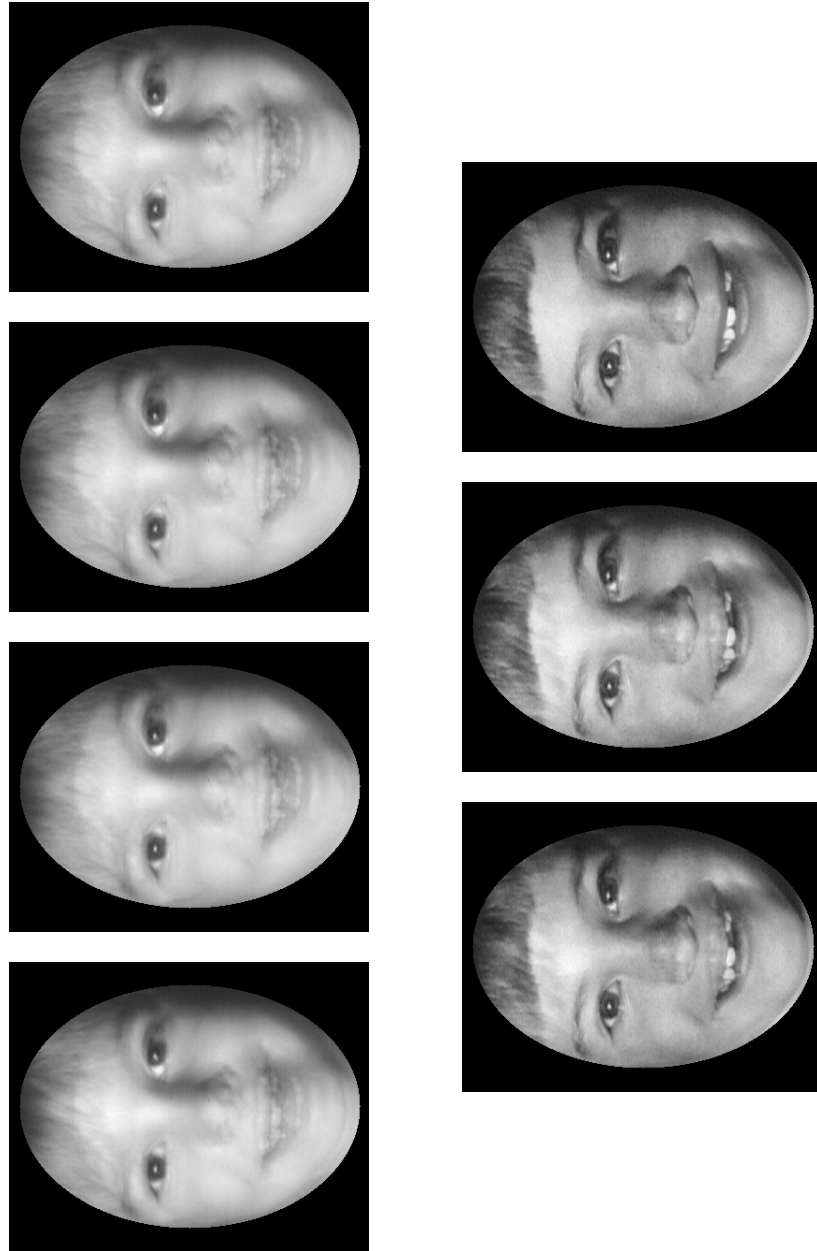
Fig. 3.6 Eigenface reconstruction. The reconstructions consist of 10, 20, 30, 40, 50 and 60 terms from left to right, top to bottom. The picture in the bottom right corresponds to the original image.
