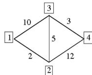
We want to consider the problem of finding the maximal data rate for sending data from node 1 to node 4. Bandwidths of all connections are shown along edges of the graph. Edges not shown have a zero bandwidth.
