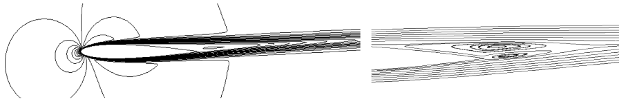
Fig. 6. Compressible flow at M = 0.5 , Re = 5000 , \alpha = 3^\circ around the NACA0012 airfoil: Mach isolines (left); streamlines near the trailing edge (right).
